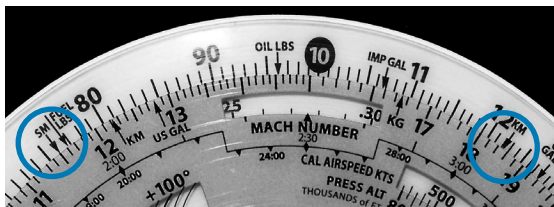
Figure 5. Set the SM value under the SM arrow and read the corresponding KM value under the KM arrow.
