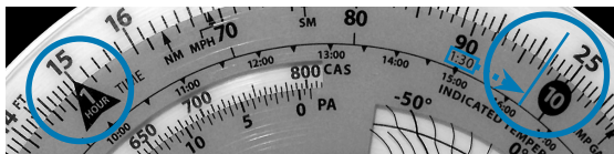
Figure 9. Place time index under ground speed then read time en route under distance.
