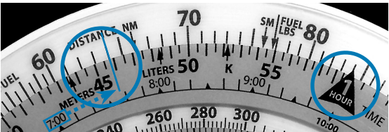
Figure 12. Point rate index to fuel consumption, find fuel capacity on outer scale and read fuel endurance below.
